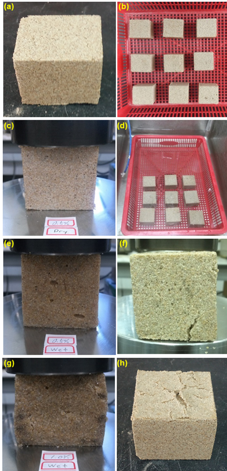
Fig. 2. Specimen conditions (a) 1st cycle; (b) drying samples; (c) UTM measurement on dry condition; (d) sample wetting (submergence) for 24 h; (e & f) before and after loading of a dry specimen; (g) loading of a 10th wet specimen; (h) Dry specimen after 10 cycles of wetting and drying.
