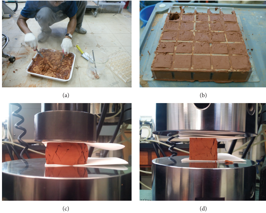
FIGURE 3: Experimental program. (a) Biopolymer-soil mixing. (b) Mixture molding. (c) UTM after 1 day of curing (ductile). (d) UTM at 28 days of curing (brittle and strong).
